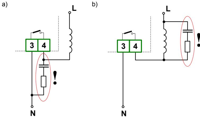
Figure 4.8. Examples of suppression circuit connection:
