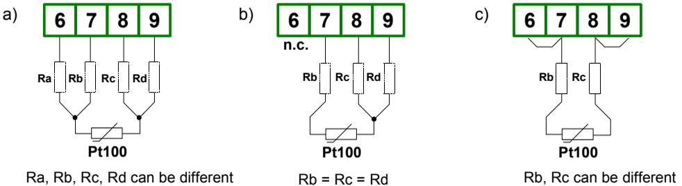
Figure 7. Connection of sensors:
